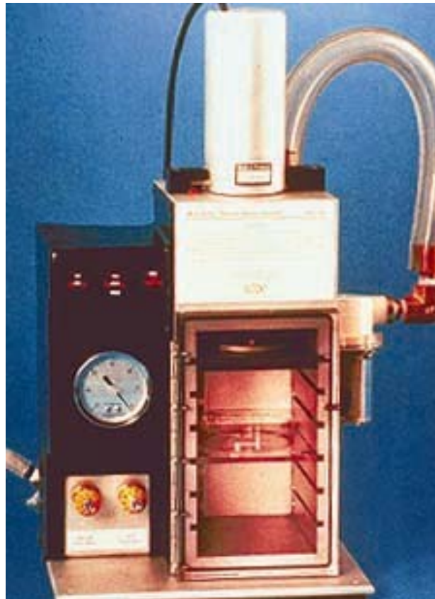
Figure 6: The "gene gun", one tool used to transform corn into Bt corn (Monsanto).
