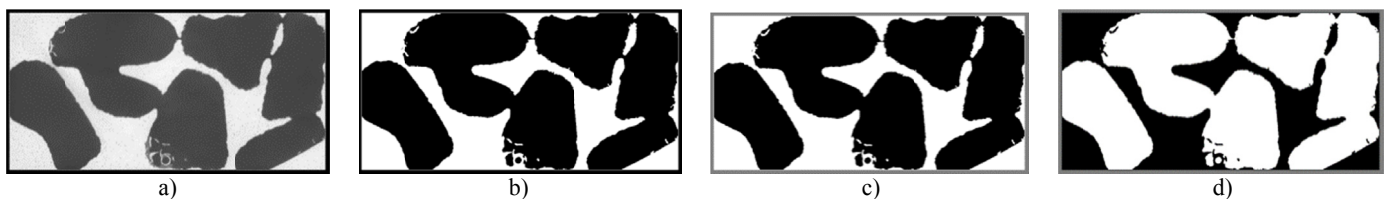
Fig. 4. From the left – (a) cropping the object, (b) binary thresholding of the image, (c) resolution of the samples and background, (d) colour inversion
