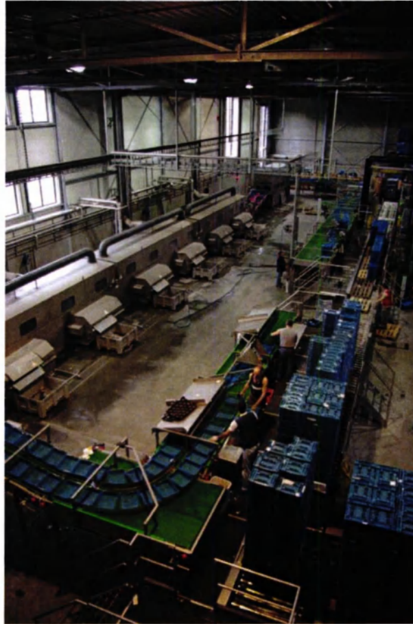
Figure 2.3. The washing installation of Euro Pool System in Geldermalsen.
