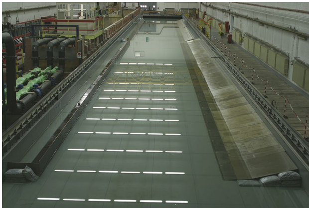
Fig. 1 Overview of towing tank with banks
