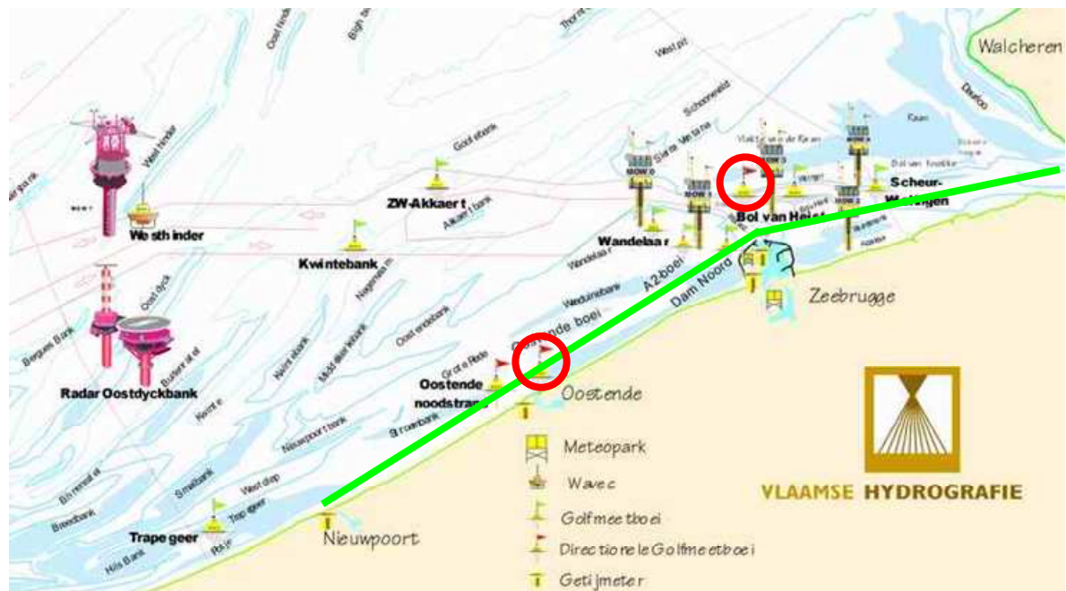
Figure 5. Measuring Network Flemish Banks (Meetnet Vlaamse Banken). Trajectories (green lines) for estuary traffic Western Scheldt – Zeebrugge – Nieuwpoort and locations of directional wave buoys (red circles) Bol van Heist and Oostende. Source: adapted from Vlaamse Hydrografie.
