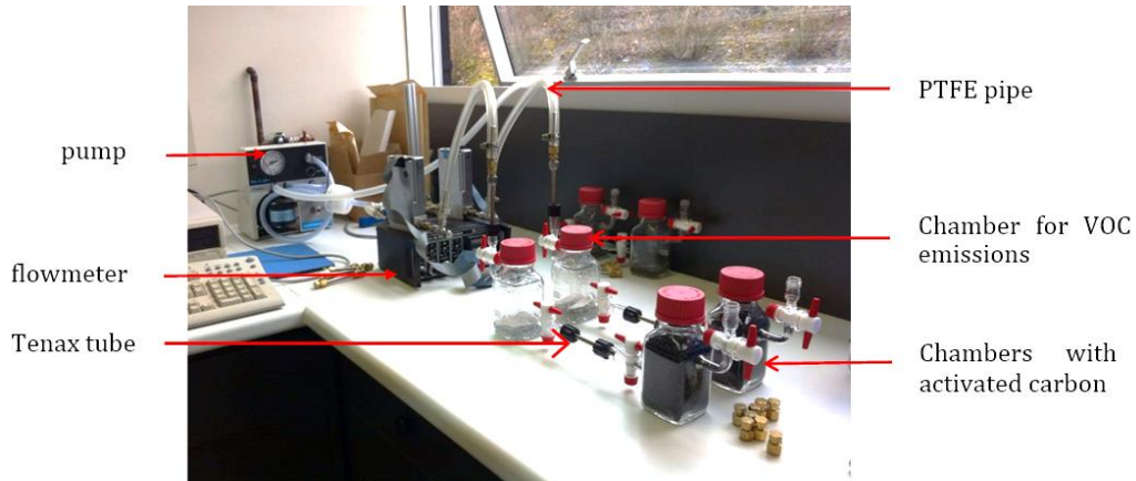
Figure 19: Experimental setup dedicated to collect the VOCs emitted during fungal development
