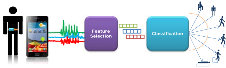
Figure 3: Activity Recognition process pipeline.
