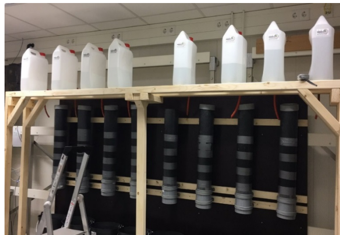
Fig. 2 Picture of experiment equipment. Eight soil columns with Mariotte bottles on top of the shelf to supply tap water.
