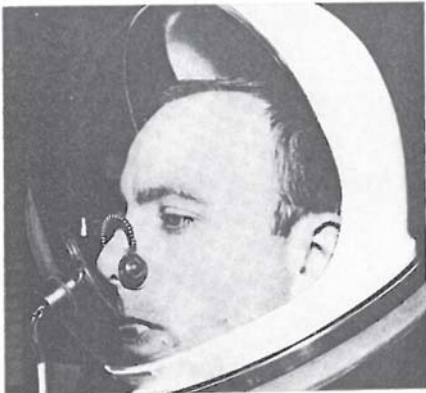
Fig. 2. Carbon dioxide monitoring in space suit research.
