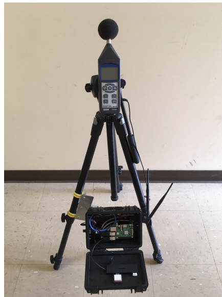
Fig. 8 Flight data system incorporating an acoustic data logger (top) and ADS-B receiver (bottom) for automated data acquisition.
