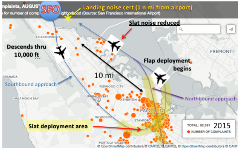
Fig. 2 Typical north- and southbound approach to SFO superimposed on a noise-complaint map [2].
