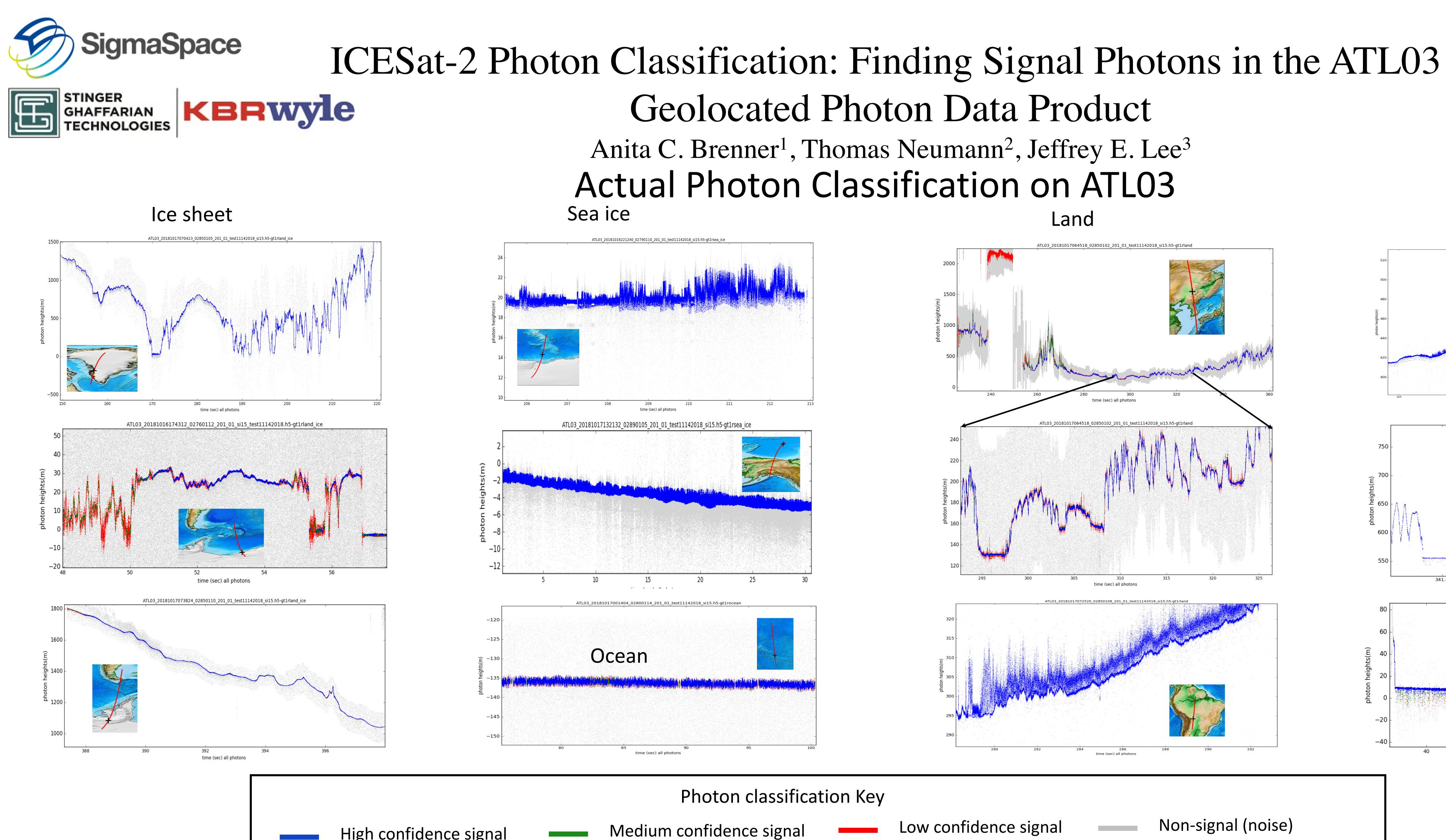
**Problem -** telemetered photon events (spanning 30m to 2000m in heights) on ATL03 contain both signal and background photon events. **Solution** - a photon classification algorithm to provide an initial discrimination between signal and background photon events. **Goal** - identify all signal photon events while minimizing false positives
