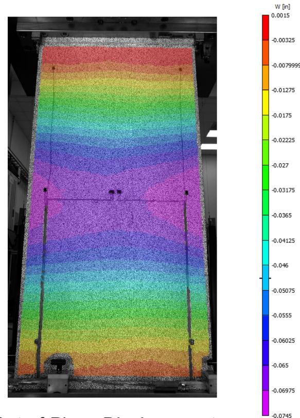
Out-of-Plane Displacement,  $w$
