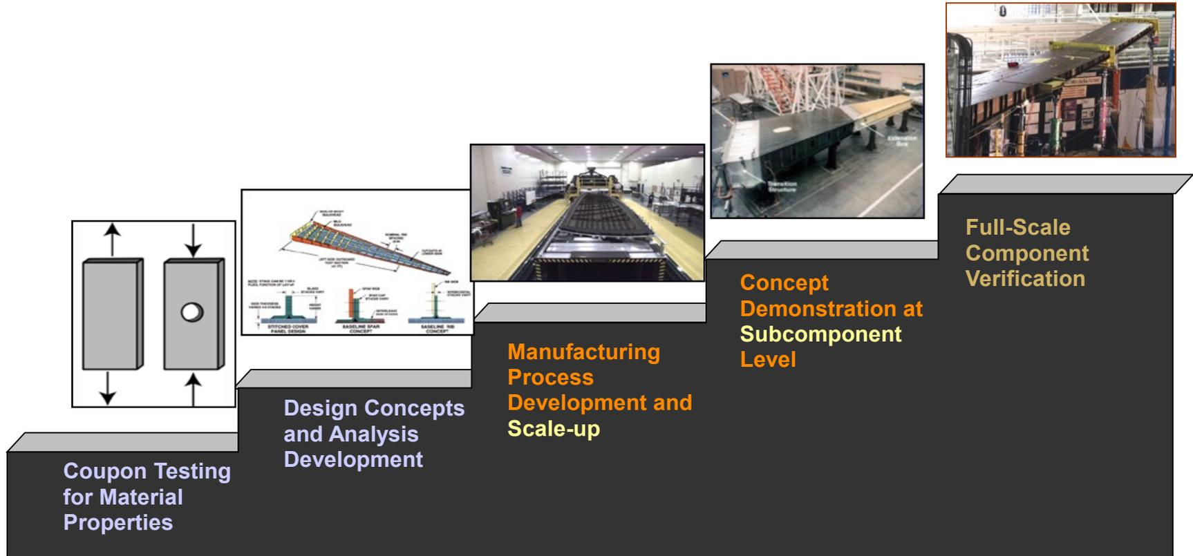
**CTE Joint design development is based on the building block approach. Scale up verification is related to subcomponent work.**
