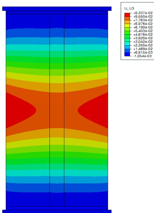
Out-of-Plane Displacement,  $w$
