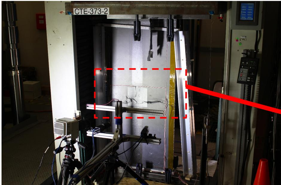
Damaged Panel at Failure
