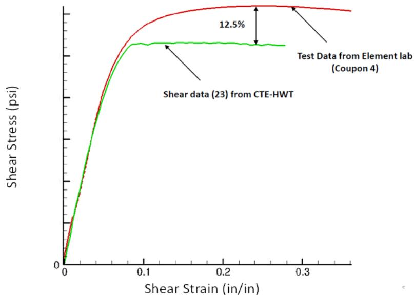
Figure 2. Comparison of analytical shear stress/strain curve to Element Labs shear stress/strain test results.
