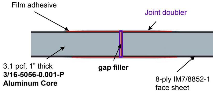
Designed L-joints and tests, verified design to 2.0 FoS
