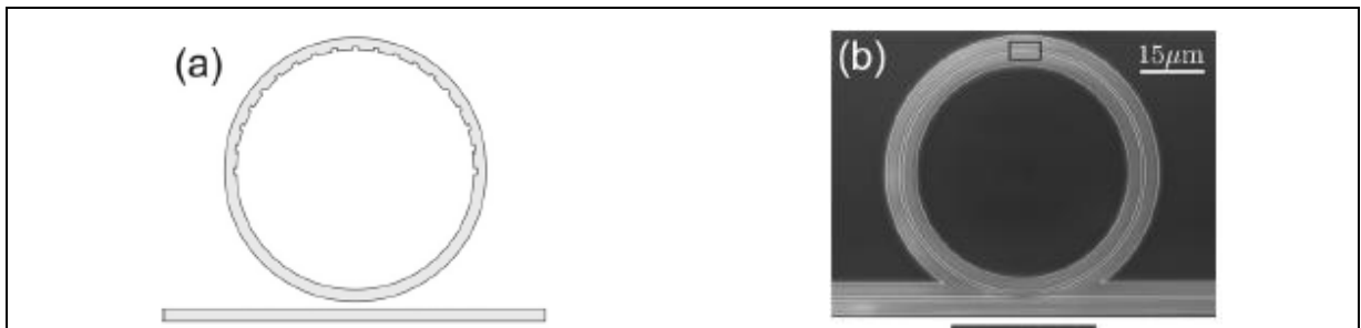
Figure 2.5 a) Schematic of the ring with integrated DBR. The DBR is realized by modulating the top half of the ring waveguide. b) SEM image of the fabricated device prior to top cladding deposition Taken from Arbabi et al. (2011)
