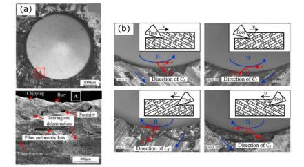
Figure 8 Exit delamination in CMCs showing (a) SEM image an exit delamination in a C/SiC material showing three different regions: tearing, edge chipping and burring (b) the influence of the fibre orientation in the delamination [33].
