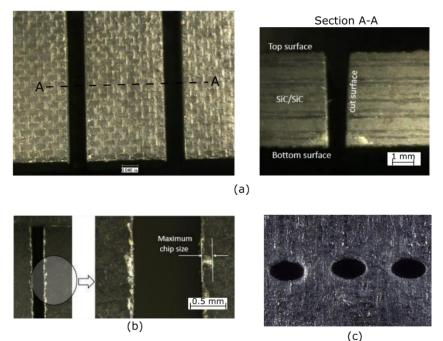
*Figure 25 Examples of (a) through cut, (b) edge fracture and (b) hole making with AWJ in a SiC/SiC material* [77].
