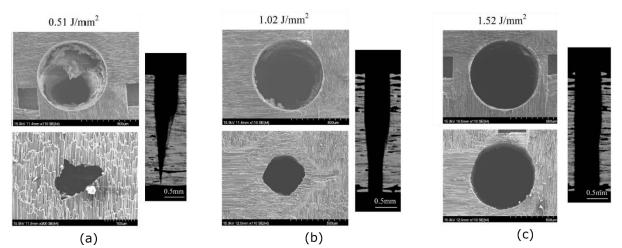
Figure 19 SEM images of the hole entry, hole exit and X-Ray CT of the hole geometry when laser-drilling a 3 mm thick C/SiC with a (a) 0.51 J/mm<sup>2</sup>, (b) 1.02 J/mm<sup>2</sup>and (c) 1.52 J/mm<sup>2</sup> [65].
