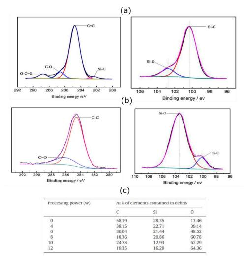
Figure 21 Surface analysis of a SiC/SiC machined with a picosecond laser showing (a) XPS spectra of the material as-received, (b) XPS spectra of the material as-machined and (c) table showing a the XPS quantitative analysis for different processing powers [62].
