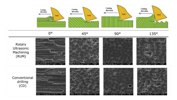
*Figure 9 Surface integrity considering different fibres orientations (0°, 45°, 90° and 135°) for Rotary Ultrasonic Machining (RUM) and Conventional Drilling (CD)* [38].
