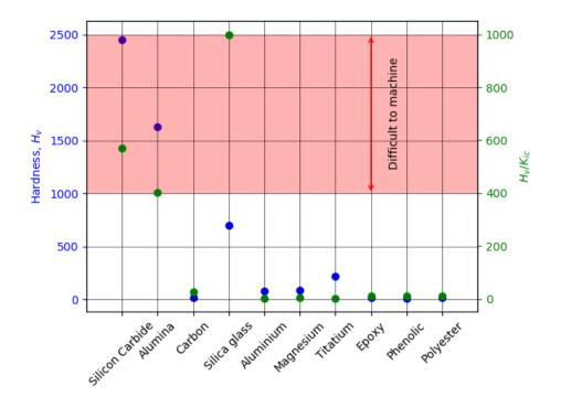
Figure 2 Approximate values from [9] of (a) H<sub>v</sub> (in blue) and (b) H<sub>v</sub>/K<sub>ic</sub> (in green) for the different materials used in the manufacturing of composite structures such as PMCs, MMCs or CMCs (red band defining "difficult to machine" has been arbitrarily drawn just to highlight the materials with higher values).
