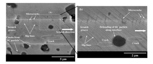
*Figure 6 (a) SEM images of the scratch induced deformation in a ZrB*<sub>2</sub>*-SiC for a load of 250 mN showing (b) slip-line patterns and micro cracks along the scratch groove* [29].
