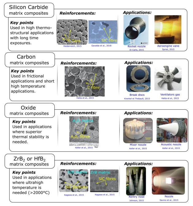
*Figure 3 Summary of the main CMCs matrices with typical reinforcements and the most popular industrial applications* [6], [7], [11]–[17].
