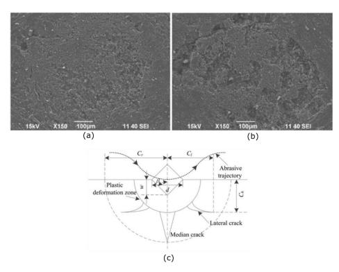
Figure 13 Surface comparison between (a) RUSM and (b) CG [45]. (c) Crack system (median and radial) in single-edge non-overlapping cut with cutting velocity directed normal to the plane of cross-section in a brittle material [43].
