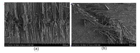
Figure 5 SEM images of a C/SiC with a scratch angle of (a) 90° and (b) 45° showing the bending mechanism of the fibres and the induced lateral damage [28].
