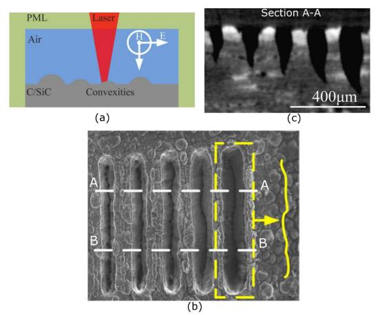
Figure 22 (a) Schematic showing how the convexities influence the laser beam incidence (b) trenches obtained in a C/SiC for 1 W, 100 µm defocus at different speeds and (c) Micro CT scan showing the Section A-A in (b) [68].
