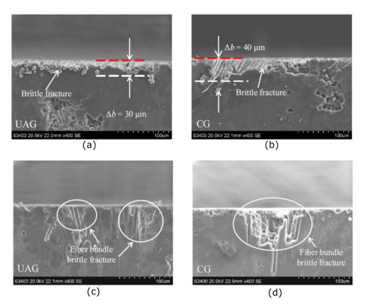
*Figure 18 SEM images of subsurface damage in 90° fibres produced by UAG and CG* [60].
