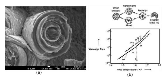
Figure 17 "Extrusion fracture" of a carbon fibre [51] probably due to its onion-skin structure and (b) different carbon fibre structures with varying melt spinning for two types of pitch [53].
