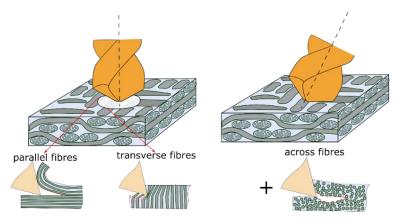
*Figure 7 Influence of the fibre orientation when drilling perpendicular and tilted holes in orthotropic material such as CMCs.*
