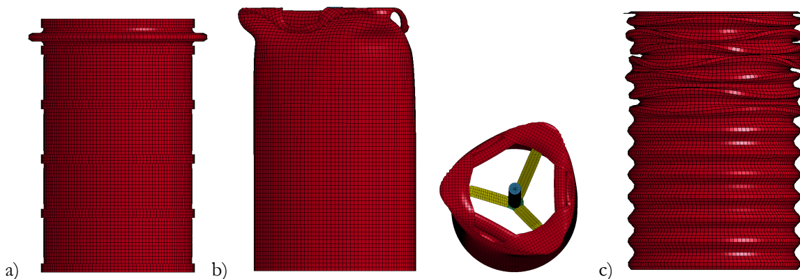
FIG 3: Deformation of different tubes after shock (a-stiffened tube, b- initiator tube, c- corrugated tube)
