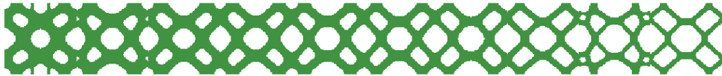
Figure 6.4: Simultaneous Optimized cells for an FGM with linear gradation in bulk modulus of elasticity.
