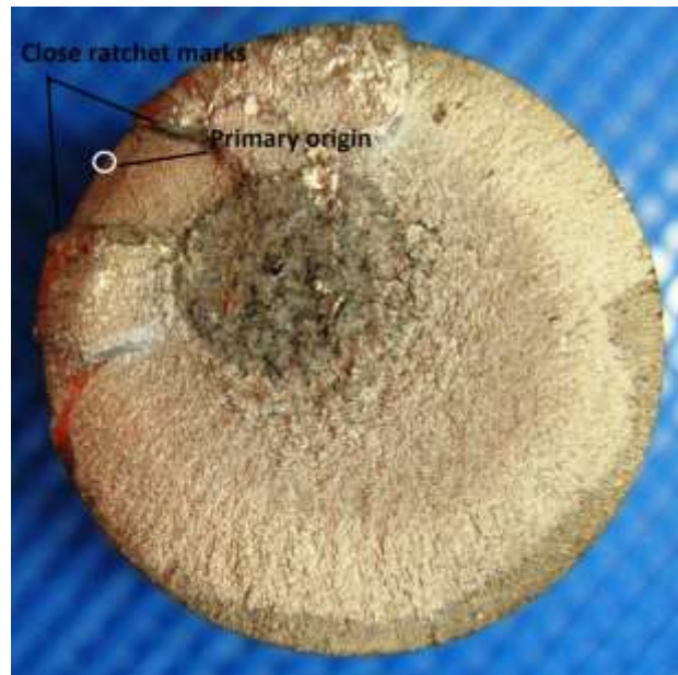
Figure 4.47: Locating of the primary origin using the angles of the ratchet marks
