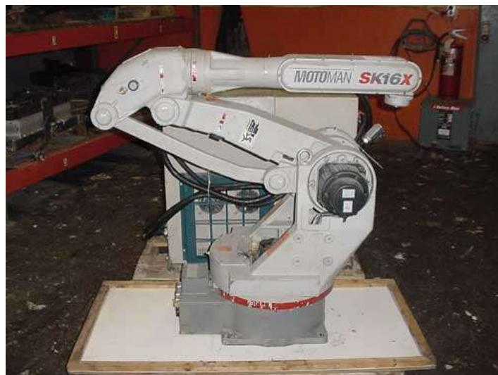
Figure 3.5: 6-axis robot used to control the laser nozzle
