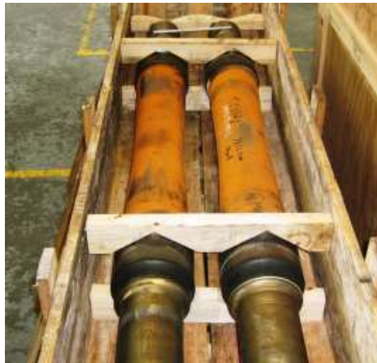
Figure 2.8: Two retired axles with corroded surface
