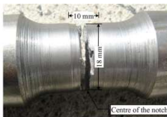
Figure 4.45: Site of fracture in a non-clad mild steel fatigue sample with an extra groove with an OD of 18 mm
