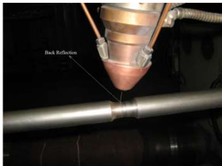
Figure 3.9: Set up of cladding head with respect to the workpiece
