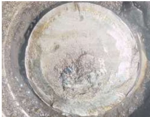
Figure 2.4: The fracture surface of an axle broken due to the fatigue failure [16]
