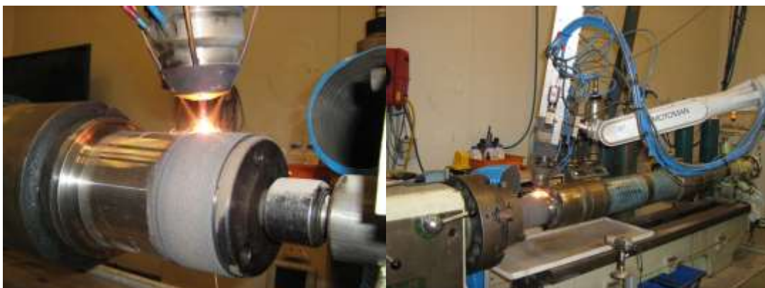
Figure 1.3: Laser Cladding of a worn railway axle in Hardchrome Engineering Pty Ltd
