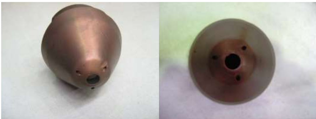
Figure 3.6: Coaxial laser heads
