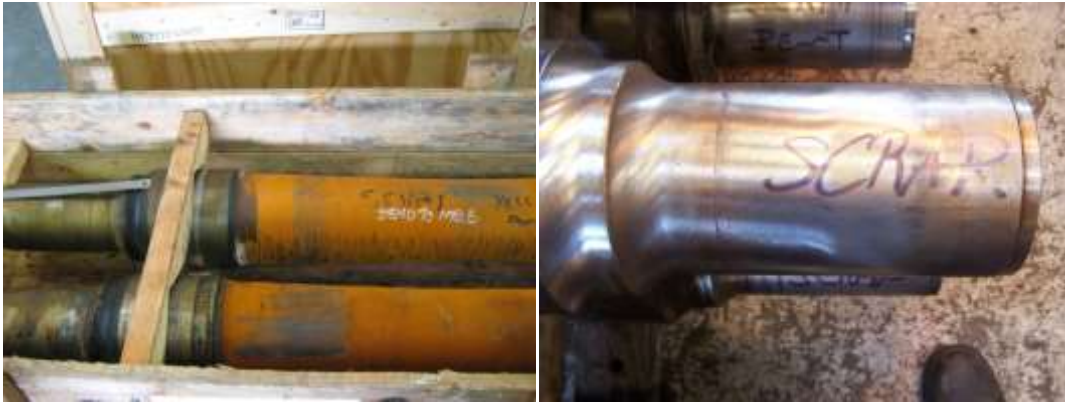
Figure 1.1: Scrapped railway axles with worn journals
