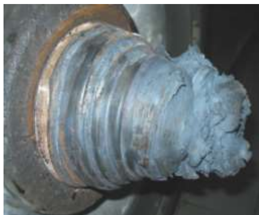
Figure 2.5: An overheated railway axle [16]
