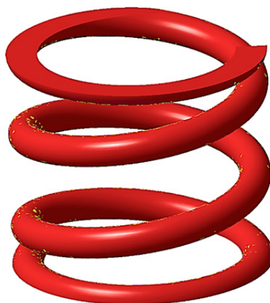
Figure 4.11 - Comparison of original and meshed spring geometry. Light shade indicates a difference of mesh geometry from original by 50.00 \times 10^{-3} mm (smallest tolerance used in simulation)
