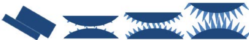
Figure 4. Illustration of particle contacts with different surface structures. (Raula et al. 2009, modified from the original).
