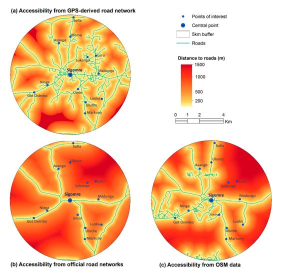
**Figure 7.** Accessibility surfaces as computed from Euclidean distance from (**a**) GPS-derived road networks (**b**) official road networks and (**c**) Open Street Map road networks.
