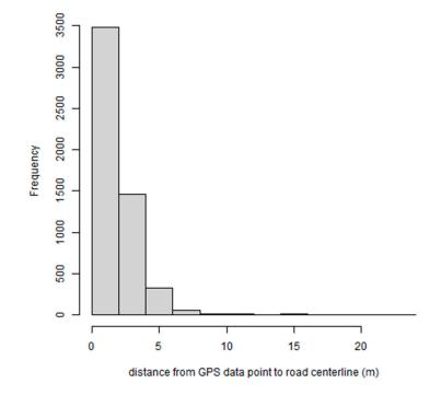
**Figure 5.** Distribution of distances between GPS data points and the centerline of official road sections in the validation section.
