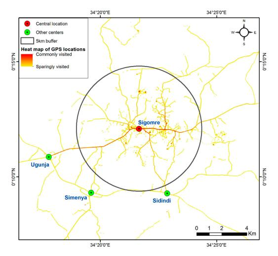
**Figure 6.** Traces of road network as visualized from the heat map resulting from the GPS traces of motorcycle taxis.
