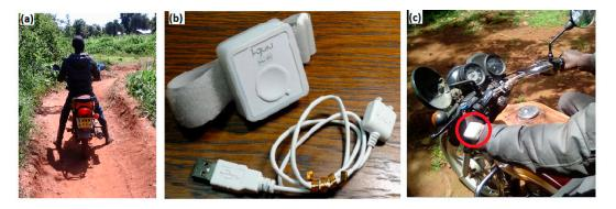
**Figure 2.** Illustration of (**a**) Typical rural motorcycle tracks (**b**) i-gotU GT-600 Global Positioning System (GPS) travel and sports data logger (**c**) A motor cycle rider strapping a GPS data logger on the wrist while riding a motorcycle taxi.
