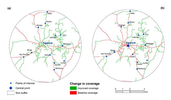
**Figure 9.** Potential improvement in map coverage of GPS-derived roads when compared against (**a**) data from official sources and (**b**) OSM tracks.
