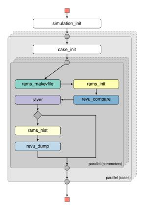
Fig. 2. Workflow of MeteoAG using the Regional Atmospheric Modelling System (RAMS) and supporting software REVU (extracts variables) and RAVER (analyses variables).
