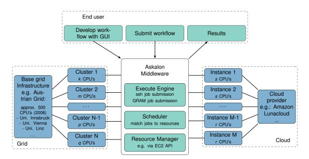
Fig. 1. Schematic setup of the computing environment for Cloud and Grid computing.
