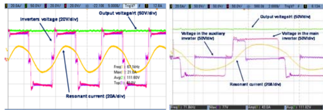
Fig. 12. Experimental measurement of a critical point: 1kW at 8kV. On the left, the minimum V_{IN}=40V requires maximum d1 and d2 to obtain full power. On the right with V_{IN}=75V one of the inverters works with lower duty cycle. The current peak is around 21A in both cases, as the model predicted.
