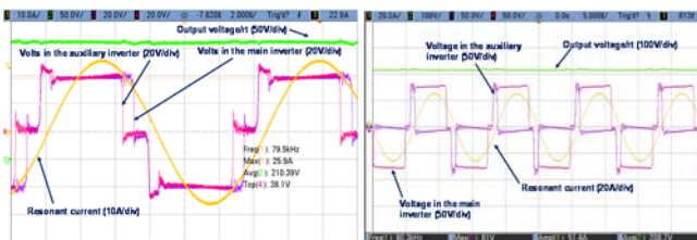
Fig. 14. Experimental measurement at 1kW, 15kV. On the left V_{IN}=40V requires large duty cycles in both inverters. On the right, V_{IN}=75V , only the main inverter is providing voltage. In both cases, as the model predicts, the resonant current is similar, around 25 A.
