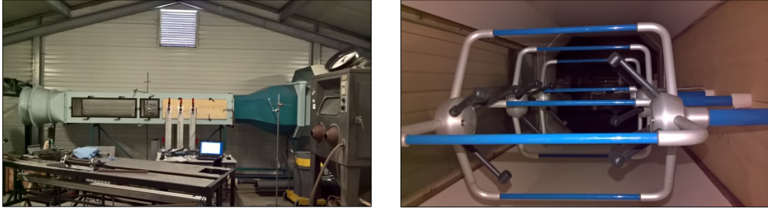
Figure 2. Details of the calibration process of the three ultrasonic 3 D anemometers in the laboratory: a) Wind tunnel and three anemometers and b) Three anemometers inside wind tunnel test section.
