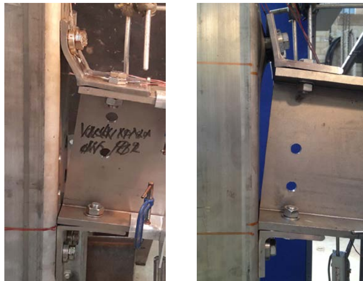
(a) TSAC-1: bending of top angle cleat
