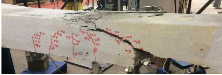
Fig. 11. Failure pattern of sleeper 3.
