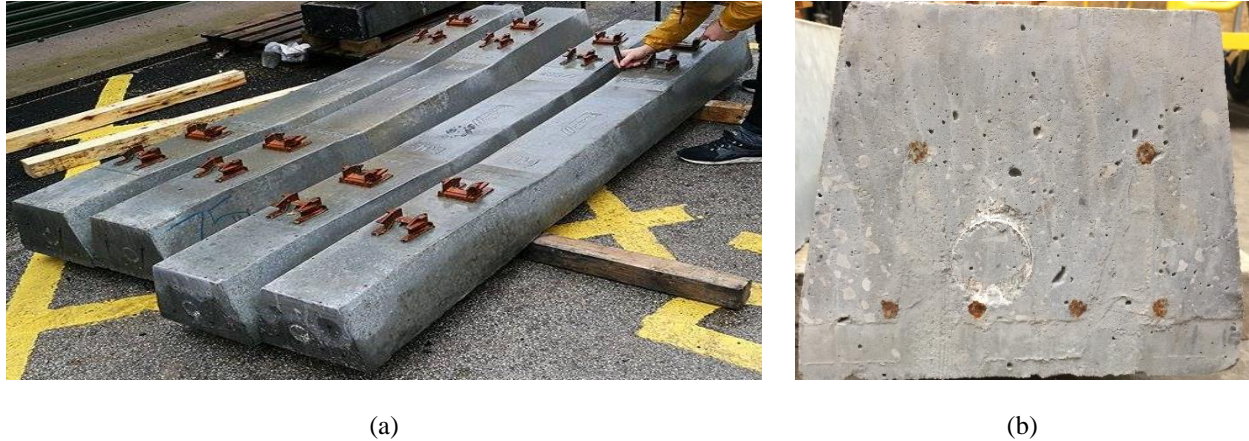
Fig. 1. Pre-stressed railway concrete sleepers: (a) four sleepers. (b) cross-section showing 6 steel tendons.
