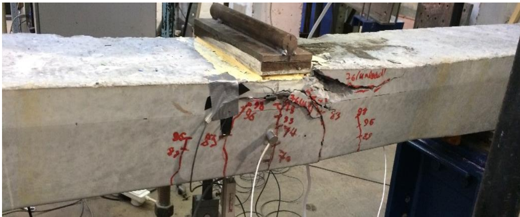
Fig. 4. Failure pattern of sleeper 1.
