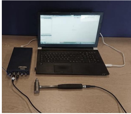
Fig 6. Impact hammer and Prosig 8004 portable acquisition.
