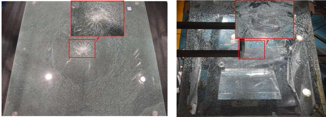
(a) Two glass crack patterns in BS3 at 1 st breakage (b) Outer glass crack pattern in BS1 at 1 st breakage
