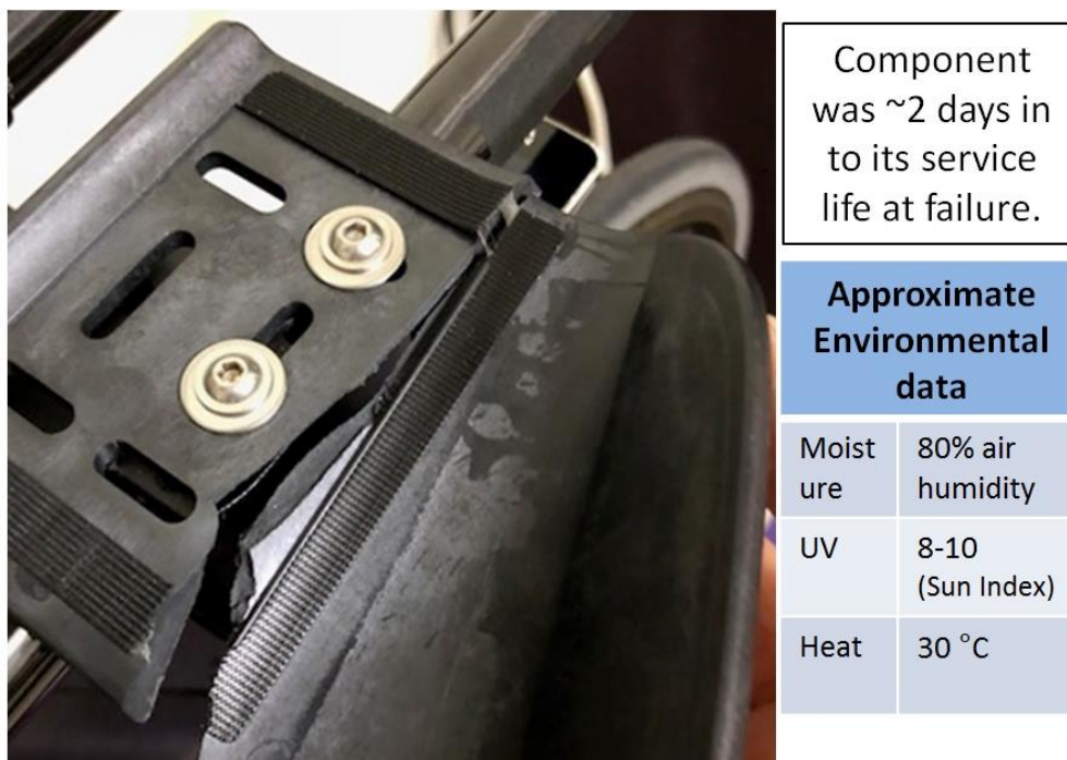
Figure 2: Fractured component mounted on the handlebars
