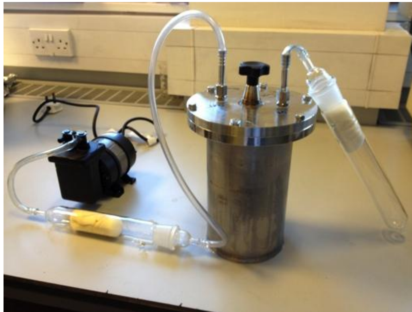
525 Figure 1: (Top) Photograph of UoB test chamber configured for experiments 526 monitoring emissions to air and (bottom) Schematic of experimental design for 527 source-air-dust transfer experiments. For UoB chamber x,y = 10 cm, for micro- 528 chamber x = 1 cm, y = 2 cm.
