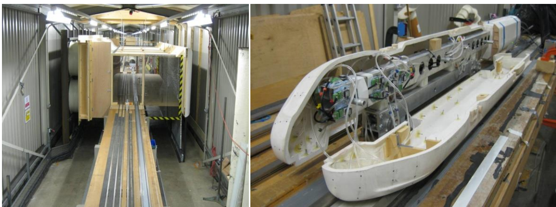
Figure 11 TRAIN Rig cross wind generator and instrumented train showing train mounted pressure transducers (28)
