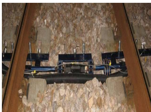
Figure 5 Pressure probes, Cobra probes (for measuring velocity) and force transducers mounted across a high speed railway track (9)
