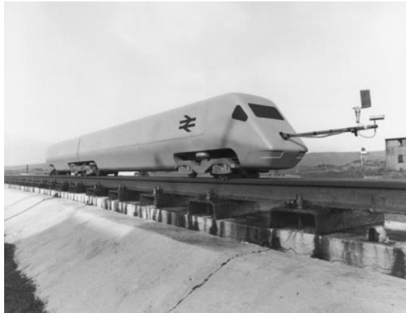
Figure 1 Measurements to measure the cross wind forces on the APT using a 1/5 th scale model at the Pendine test establishment (4)
