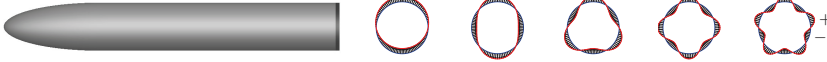
Fig. 2 Location of the distributed forcing (dark) on the trailing edge of the bluff body and illustration in the (y, z) plane of the azimuthal sine-type waveform at wavelength \lambda_\theta = 2\pi/1, 2\pi/2, 2\pi/3, 2\pi/4 and 2\pi/5 , from left to right (blue circle depicts the trailing edge section. + and - symbols indicate regions of blowing and suction respectively).
