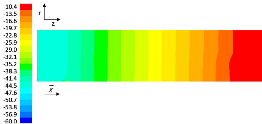
Fig. 6. Pressure field (Pa). ( q_L=16 \text{ m}^3/\text{m}^2/\text{h} , F_S=31.5\%F_C ), case b in Table 1.
