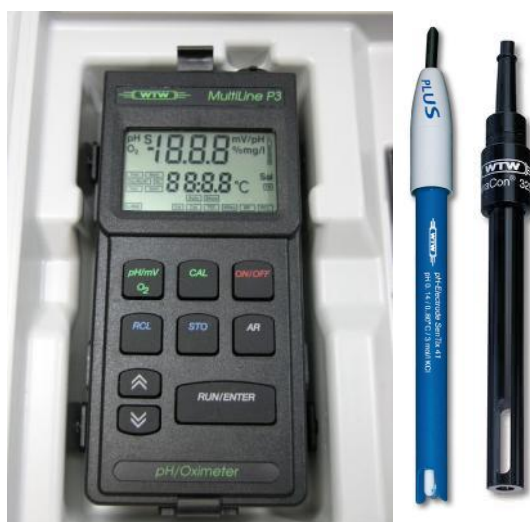
Slika 27: Multimeter Multiline P3, sonda Sentix 41 in sonda Tetracon 325
