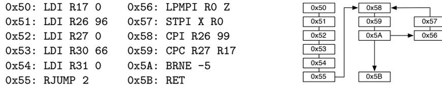
Fig. 1. An initialisation loop for the ATMEL ATmega16
