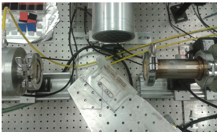
Figure 2.3: Top-down view of the sample holder and configuration of the samples with respect to the beam and detector
