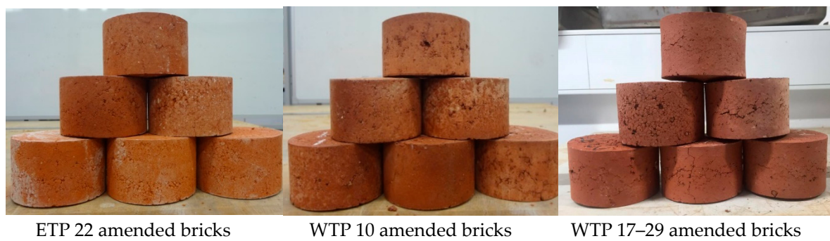
Figure 7. Samples of manufactured ETP 22, WTP 10 and WTP 17–29 brick samples.
