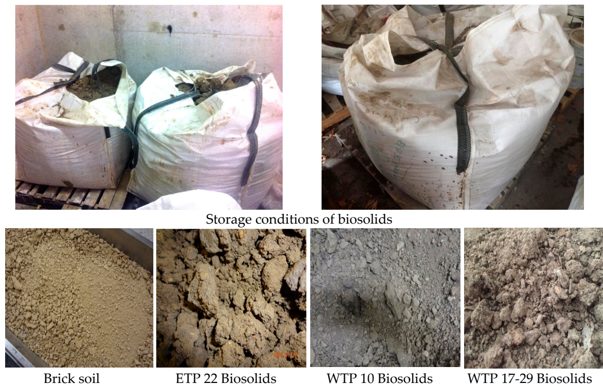
Figure 2. The storage conditions of the biosolids and close-up views of each sample.
