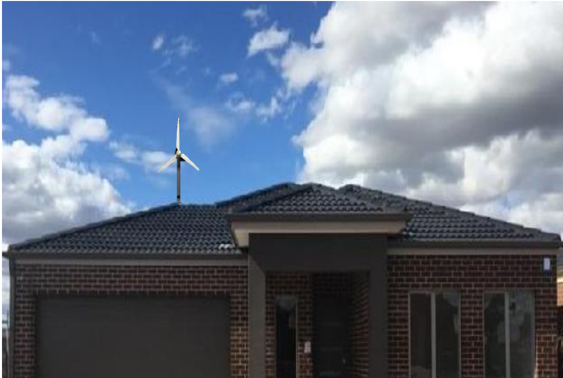
Figure 1.26: Domestic scale horizontal axis wind turbine
