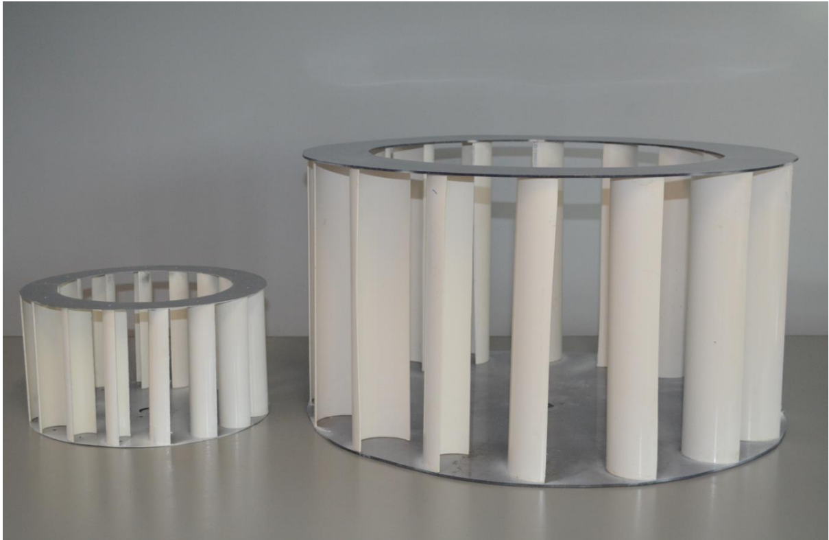
(b) Prototype 16-blade turbine
