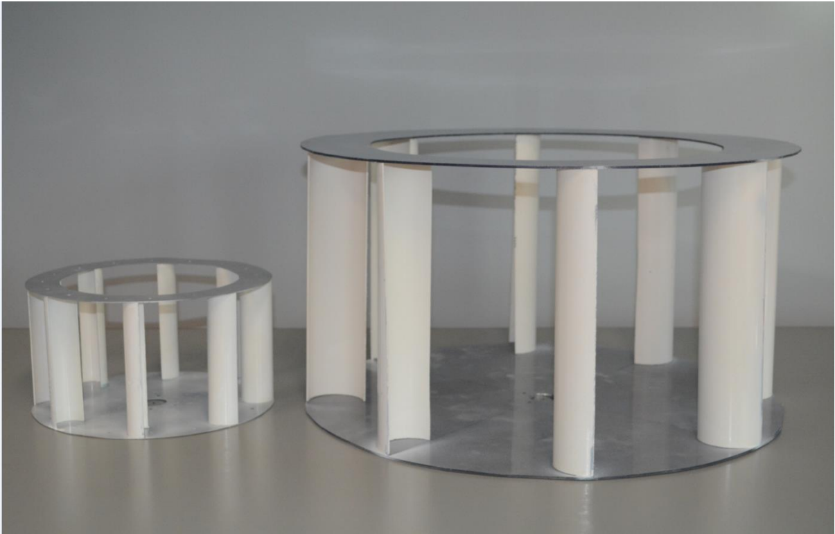
(a) Prototype 8-blade turbine
