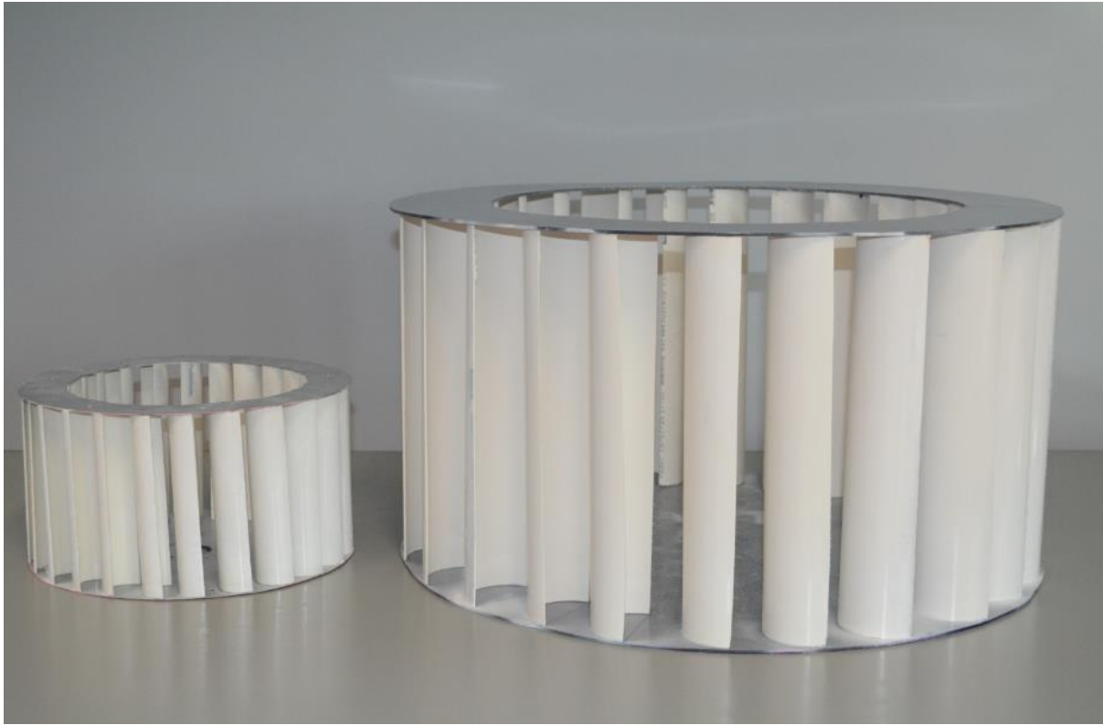
(c) Prototype 24-blade turbine
