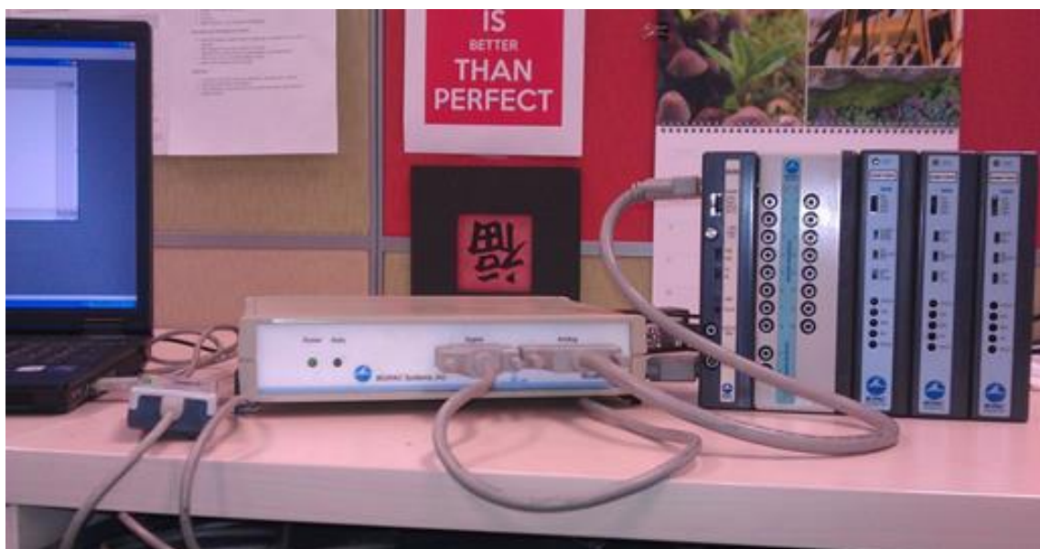
Figure 10: Biopac hardware setup Left to right: PC running AcqKnowledge, Biopac Serial to USB adapter, MP100, various Biopac amplifier modules connected to MP100 via both Digital and Analog DB cables.
