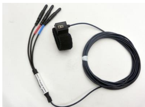
Figure 17: Biopac TSD200 PPG sensor [59]
