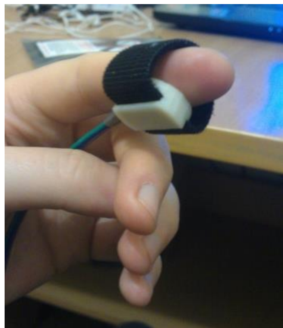
Figure 15: PPG finger showing PPG housing and Velcro attachment
