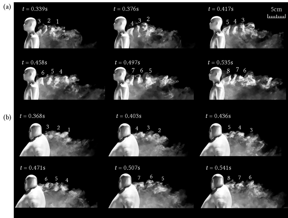
Figure 7.8 vortex shedding at the shoulder of (a) a slim body; (b) a larger body
