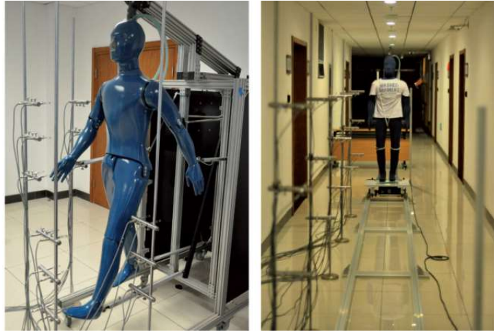
Figure 2.3 Indoor Experimental study of flow field induced by limbs pendulum and body motion measured by anemometers (Han et al., 2015)
