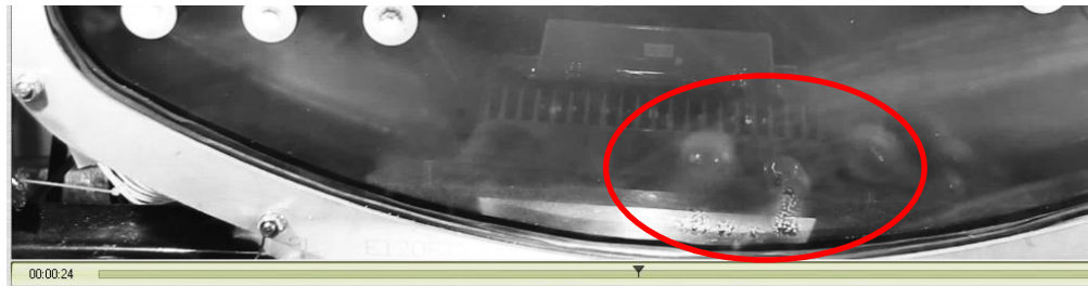
Figure 6-21: bubbles growth and merging (bed depth 32mm, q 5 kW/m 2 )
