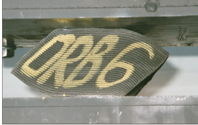
Figure 3. Fiber-reinforced strip bearing under vertical load and horizontal displacement test.
