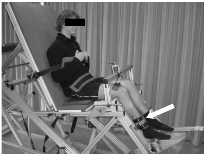
Figure 1: Lower extremity system, with the white arrow indicating the location of the force transducer
