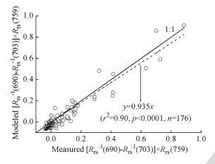
Fig. 8. Comparison of measured and modeled  $[R_{rs}^{-1}(690) - R_{rs}^{-1}(703)] \times R_{rs}(759).$
