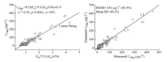
Fig. 9. Retrieval model of Chla concentration and comparison of measured and estimated values using the band-ratio method (44.4% in the bracket is the percentage of RMSE accounting for the mean  $C_{Chla}$ ).
