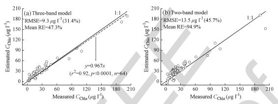
Fig. 10. Comparison of measured and estimated Chla concentration ( $C_{Chla}$ ) of the three-band model and band-ratio method based on an independent data set (31.4% and 45.7% in the bracket are the percentages of RMSE accounting for the mean  $C_{Chla}$ ).
