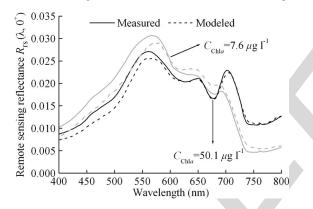
Fig. 5. Comparison of measured and modeled remote-sensing reflectance just above the water surface  $R_{\rm rs}(\lambda, 0^+)$  from two sites in July 2006.
