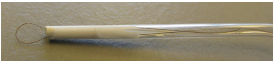
Figure 2. Hair loop tool. A piece of human hair is inserted as a loop into the opening of a Pasteur pipette and fixed in place with super glue or with Tipp-Ex. This provides a convenient tool for gently manipulating fragile zebrafish embryos.
