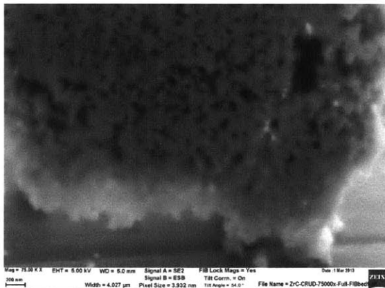
14)d) ZrC at magnification x75,000 showing the CRUD-ZrC interface.
