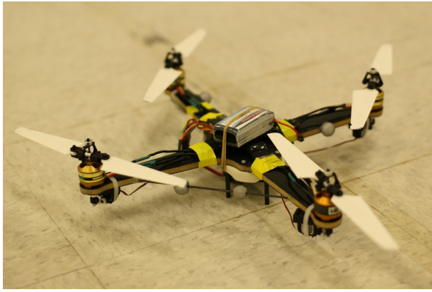
Figure 1. Variable-pitch quadrotor designed at the Aerospace Controls Lab. The servos that actuate the variable-pitch propellers are visible under each of the motors. The quadrotor measures 0.35 m across.
