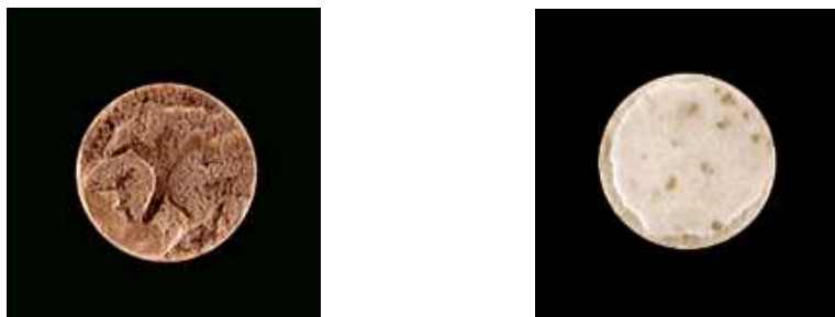
Fig 9 – Examples of Capping (at the left) and Sticking (at the right), ecstasy database IPS-WD.
