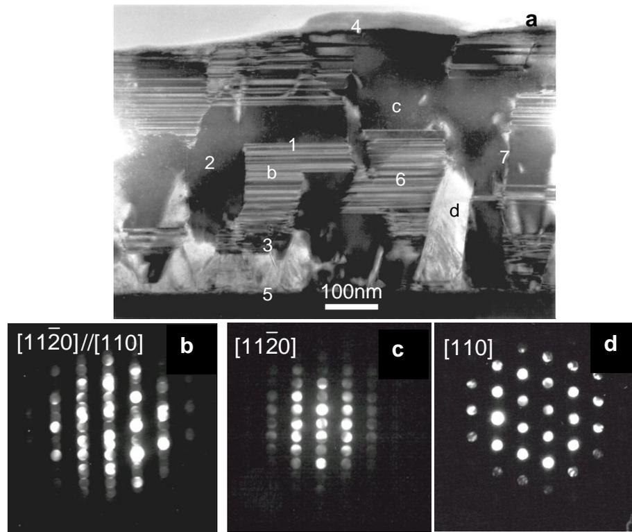
**Figure 1.** Focused probe diffraction patterns obtained from the areas labelled in (a) the bright field image for (b) a region containing stacking faults; (c) the wurtzite GaN $\langle 11\bar{2}0 \rangle$  matrix and (d) a zincblende GaN $\langle 110 \rangle$  grain.
