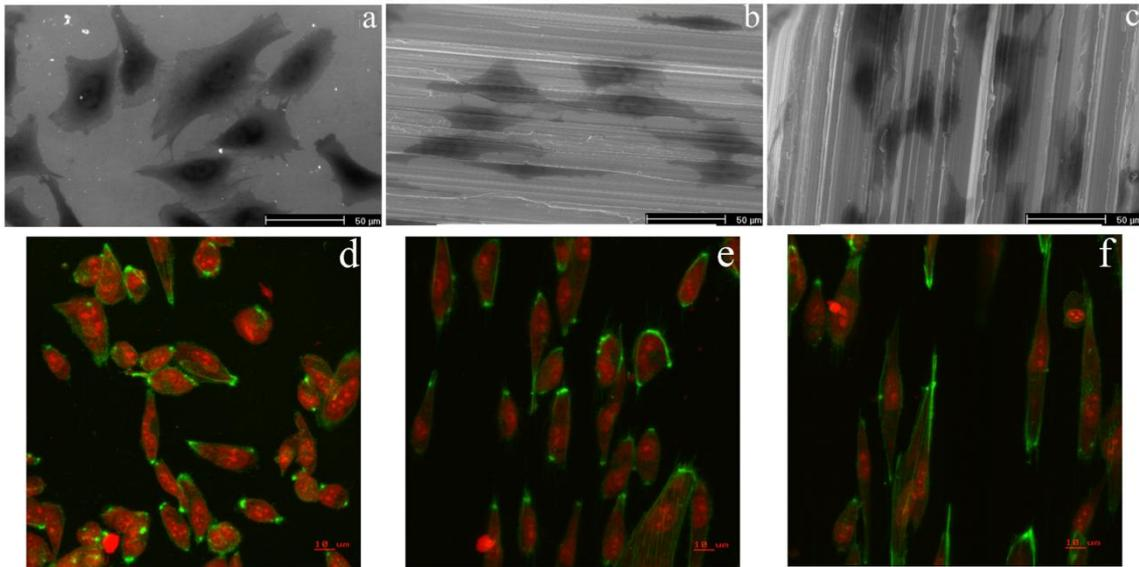
Figure 3: ESEM (a-c) and CLSM (d-f) of HOBs culture for 6 hours on stainless steel surfaces (a,d) polished; (b,e) roughened with P80 SiC and (c,f) roughened with P40 SiC paper.
