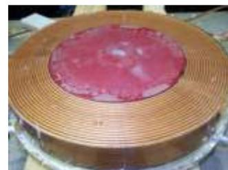
Figure 1: The insert coil.
