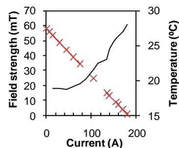
Figure 3: Net magnetic field strength (crosses) near the coil surface as current is ramped from zero to full design value. Steady-state temperature (solid line) was measured at coolant outlet.
